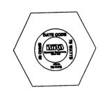
SPECIFICATIONS: POWER RATING 75 W MAX. @ 40°C. 90 W MAX. @ 25 C. FREQUENCY RANGE & VSWR: DC TO 1GHz AT 1.10:1 MAX. 1GHz TO 4GHz AT 1.25:1 MAX. IMPEDANCE: 50 DHMS, NOMINAL AMBIENT TEMPERATURE RANGE: -40°C TO +40°C CONNECTOR: TNC FEMALE (SILVER OR TRI-ALLOY PLATED) OPERATING POSITION: ANY (CONVECTION COOLED)
